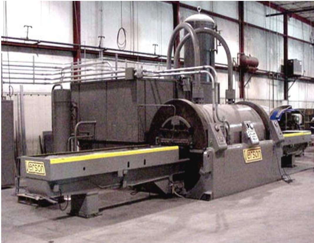
Verson Wheelon 16200R 36-120 Fluid Form Press. Tray size: both 36"x120" with bottom depth of 4 ½" and 6 ½". Capacity Tonnage – 16,200. Pressure Forming – Maximum psi 7,500.
